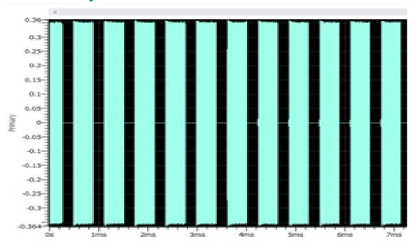
Synchronous captured Tx13 mode. X-axis is time in msec Y-axis is Amplitude in volts
