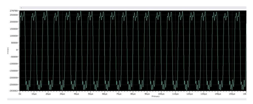
GFSK demodulated waveform. X-axis is Time in usec Y-axis is frequency deviation value in Hz.
