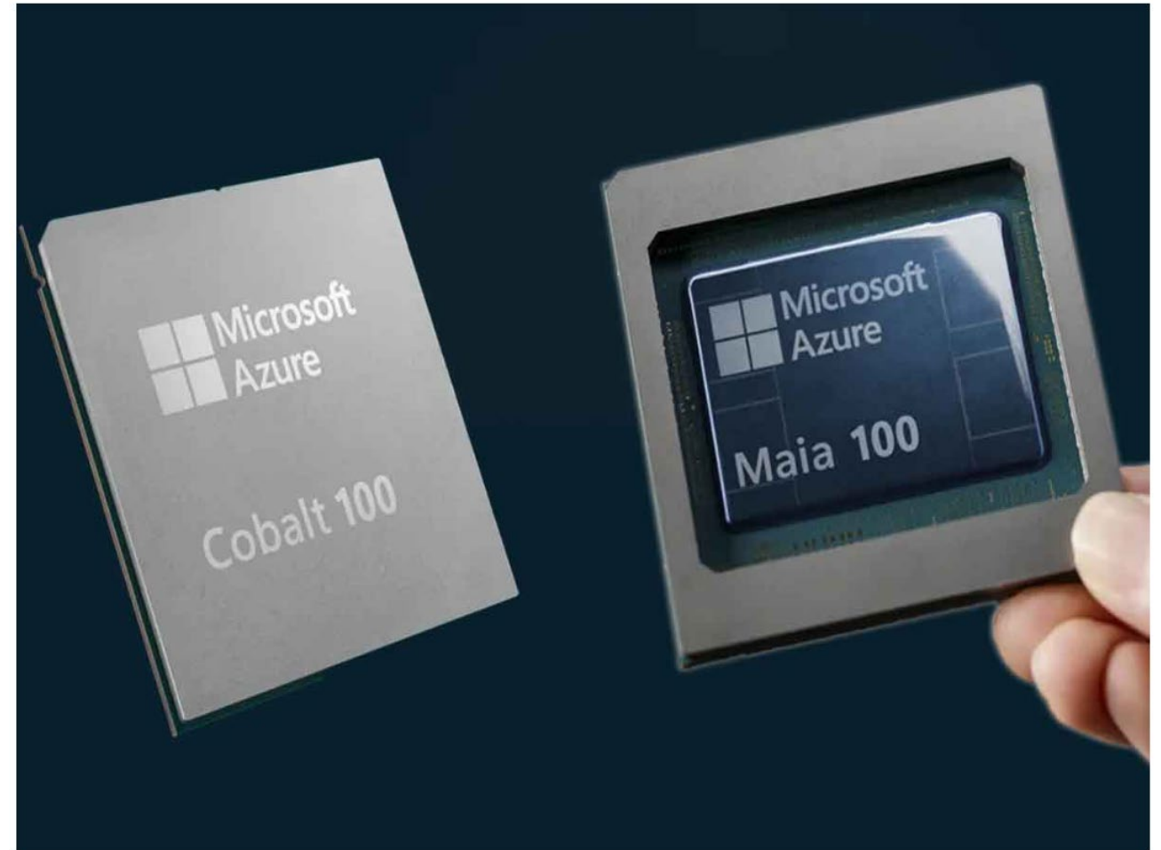
The Azure Maia 100 and Cobalt 100 chips mark Microsoft's debut into custom silicon tailored for its cloud infrastructure. / Microsoft
